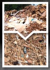
Processing waste wood of categories A1 to A4 for material/thermal recycling. in bio-power plants.
